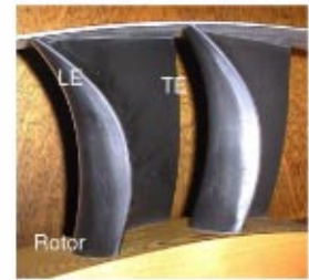
Fig. 2 (a) Large-scale rotating delta wing in the turbine rig, (b) stator vane, (c) rotor blade
